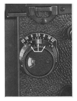
The depth of field for a given aperture and camera-to-subject distance can be read off the depth-of-field scale around the Focusing Knob. By checking this scale, you can easily determine before shooting the extent over which the objects will appear sharp and clear...
