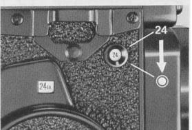
1b. When the figure "24" appears in the exposure counter window, it signifies that the full length of the film has been exposed. Another wind of the crank-handle will bring out the Mark in the window, but continue winding until the crankhandle turns freely without tension.
