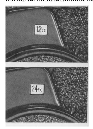
When the back cover is closed, the exposure load reminder window will show "12 EX" (green) in case of 120 film, and "24 EX" (red) in case of 220 film, to check the exposure load of the film in use.
