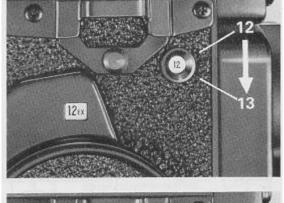
1. When the figure "12" appears in the exposure counter window, it signifies that the full length of the film has been exposed. Another wind of the crank handle will set the exposure counter between "12" and "13", but continue winding until the crank-handle turns freely without tension.
