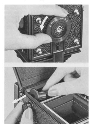
1. The Back Cover will spring open when the Back Cover Locking Ring is turned in the direction of "O" (Open).
