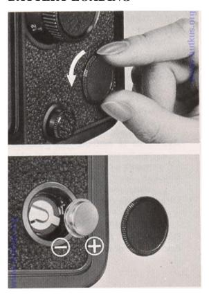
1. Open the Battery Compartment Cover holding with finger and by turning it counter-clockwise. This camera uses a 1.3 V mercury battery to power its exposure meter. Use either Mallory PX-13B, Eveready EPX-13 or equivalent.
