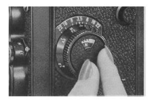
After loaded the film, turn the Film Type Indicator as illustrated, so that the letters equivalent to the film type in use are indicated in the window.
